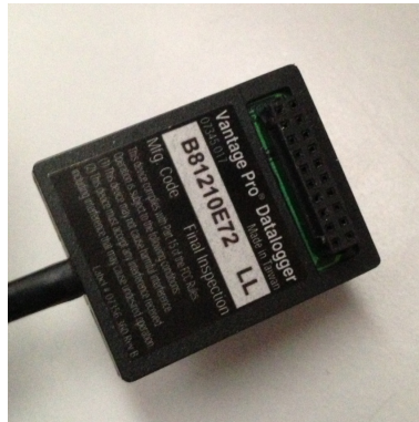
Figure 1: Original Davis data logger — non-green dot version (product # 06510 SER).
