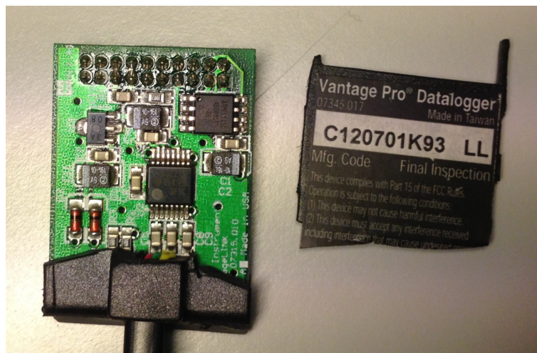
Figure 2: Original Davis data logger, under the cover — green dot version (product # 06510 SER).
